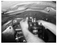
**7.** Remove the three upper strut mounting bolts with a 14 mm ratchet.
